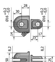
Alu/Stainless steel with clevis Max. static load 18100 N
