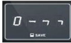
Figure 5: The key indicates that the keylock is enabled
