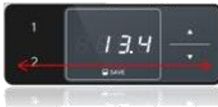
Figure 6: Activating and deactivating the keylock can be done by swiping left or right underneath the display
