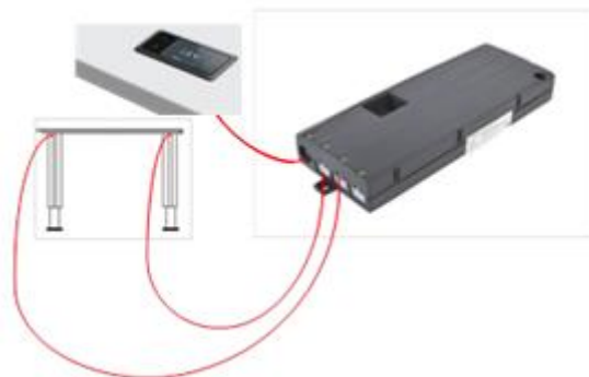
Figure 3: Connection of the TOUCH-IL to a COMPACT eco control unit
