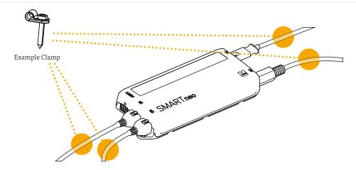
Fig. 5: Positioning the Cable Clamps
